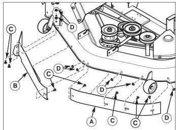
Figure 3. Blowout Baffle Installation
